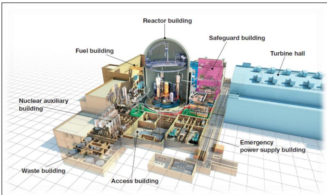
*A cutaway view of ATMEA1 reactor and adjacent buildings*
