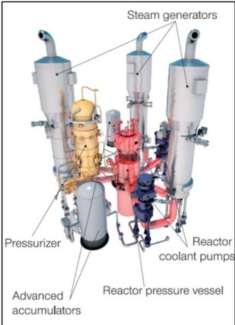
The ATMEA1 reactor's primary system configuration (a third reactor coolant pump is not visible because of the pressurizer)
